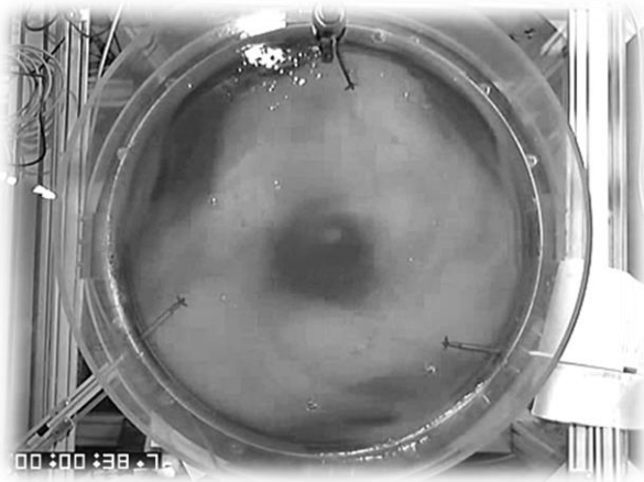
Fig. 12. Flow field at a xanthan gum of 2 g/kg (stirrer speed: 3000 rpm; azimuth angle: 65°)
